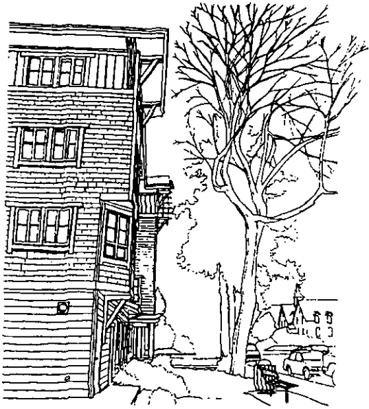
Figure 42: Building Materials (b) (v). The architectural detail and varied materials demonstrate quality design and reduce the scale of this four story residential building by clearly articulating the bottom, middle and top.
