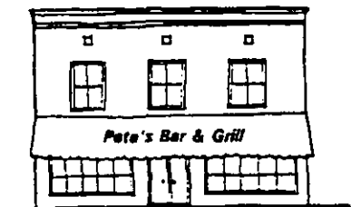
Incorporate sign as part of building element such as awning or canopy
